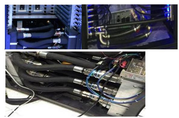
Fig. 2. Liquid Cooling Connections Using Quick Connect Couplings from Andrew Wasielewski (iPhone), CEJN, 3 Dec. 2015.
